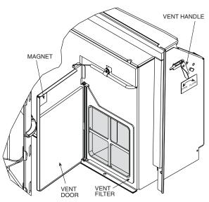
FIGURE 18 — OUTDOOR VENT FILTER (Left Side of Chassis)
